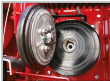
CONTROL YOUR SPEED Variable speed disc drive transmission.
